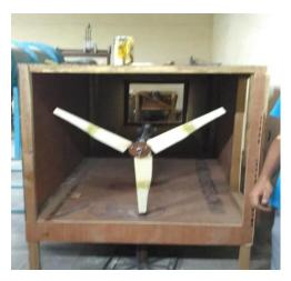
Fig 4: 3-D Printed Blades in wind tunnel
